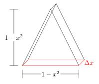
We know the cross section is an isosceles triangle where the base is equal to the height. (We actually do not need the information that the triangle is isosceles, since its area only depends on the base and height.) The area of a triangle is one half the product of the base and the height, and to find the volume of this slice we multiply that area by the thickness,  $\Delta x$ . So,
