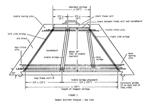
The longest string will be 35", divided by a bridge that separates the string into 14" and 21". The left section of the string should produce the note G#3, and the right section C#3. The frequencies of these notes are 207.65 Hz and 138.59 Hz, respectively. I wanted to calculate the tension needed on this first string to produce these notes, but
