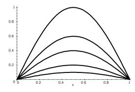
Temperature behavior in the rod starting from  $\sin(\pi x)$ . The temperature drops gradually until 0 because the second derivative of u is negative (u is concave).
