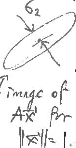
Length of semi-minor axis of ellipse, OR, Min. dist. of any  $Ax$  from origin, for  $\|x\|=1$ .
