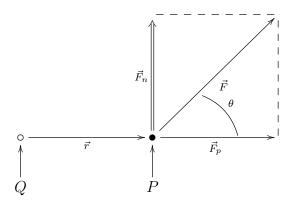
An object • (at point P) is attached by a rigid rod to a fixed point  $\circ$  (point Q), but is free to rotate around that point in any direction. The vector  $\vec{r}$  goes to the object from the fixed point around which it may rotate. A force  $\vec{F}$  acts on the object.
