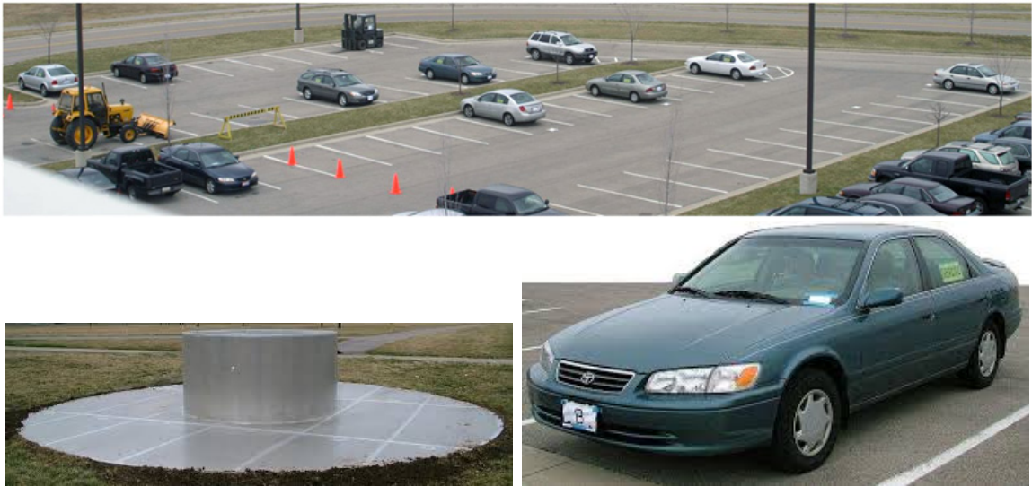
Figure 3.1: Optical images of parking lot being imaged in GOTCHA dataset. Note scene contains a variety of calibration targets, such as primitive reflectors like the tophat shown, a Toyota Camry, forklift, and tractor.
